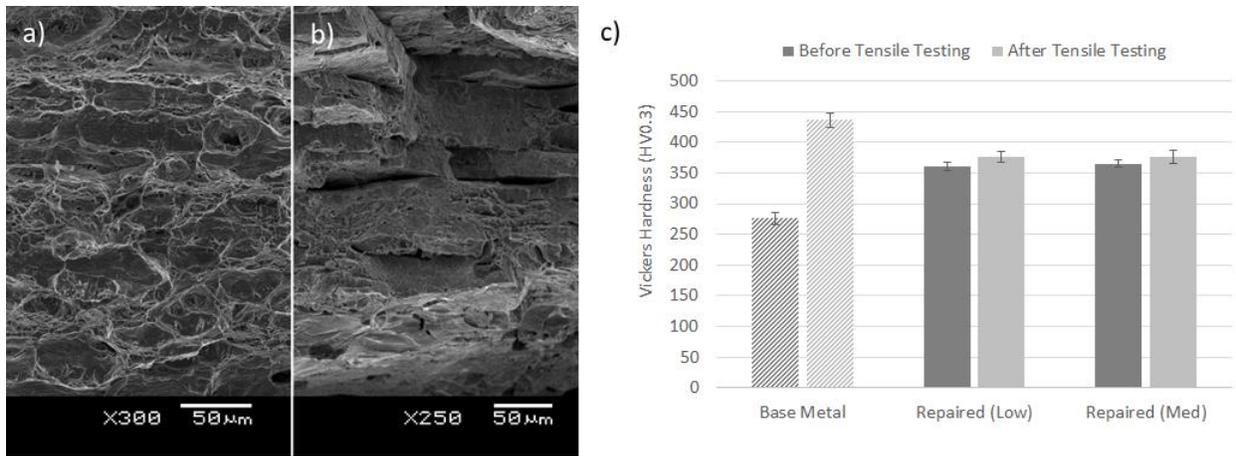
**Figure 5.** SEM image of **a)** base metal fracture surface, **b)** deposition fracture surface with step facets, and **c)** microhardness measurements and standard error of base metal and deposition in repaired specimens within 300  $\mu\text{m}$  of the fracture interface before and after tensile testing
