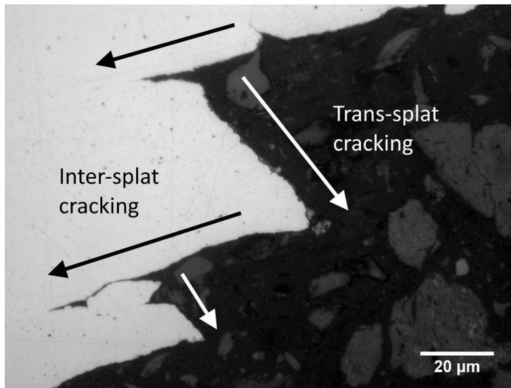
**Figure 8.** Cross sectional OM image of fracture surface showing inter-splat and trans-splat cracking
