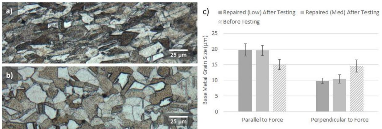
**Figure 6.** Grain structure of Inconel 718 base metal **a)** within 300  $\mu\text{m}$  of the fracture interface, **b)** as received prior to testing and **c)** the grain size and standard deviation in the base metal before and after tensile testing within 300  $\mu\text{m}$  of the fracture interface
