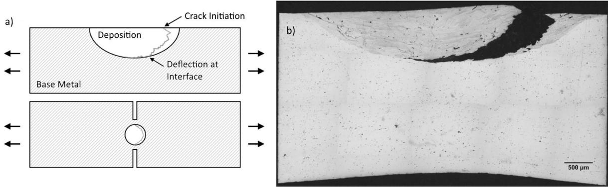
**Figure 7. a)** Side and top view schematic of crack location relative to deposition geometry and **b)** cross-sectional OM image of a lightly etched specimen tested until the initial fracture of the deposited material
